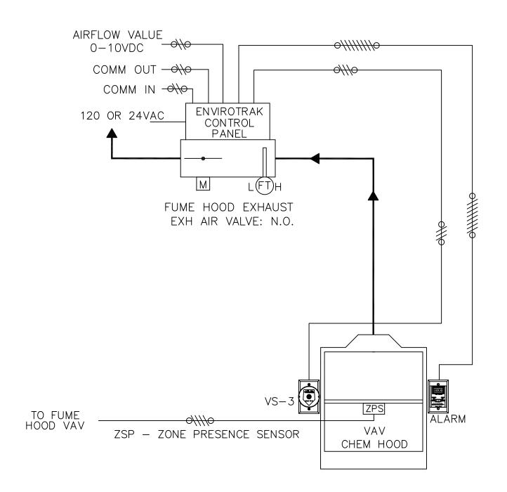
AIRFLOW AND FIELD WIRING DIAGRAM
