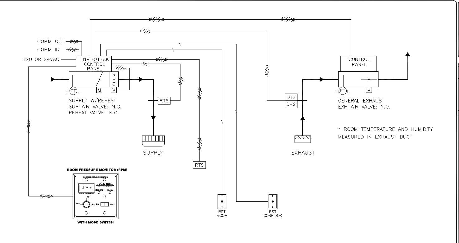
1/4" PNEUMATIC TUBING FURNISHED, INSTALLED AND TERMINATED BY ATC 2 CONDUCTOR CABLE FURNISHED, INSTALLED AND TERMINATED BY ATC
